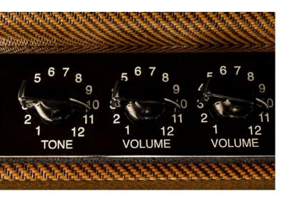
The interesting thing about the two Volume controls is that they are interactive — the Volume control of the Channel you are not plugged in to has an effect on the response of the Channel you are plugged in to.
