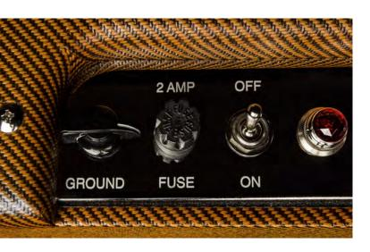
Located next to the Fuse Holder is the VAC control (GROUND). This is a built in attenuator. Its purpose is to allow the Volume controls to be turned up to achieve the desired sound, but then reduce the overall volume level with the VAC, retaining the turned up sound.
